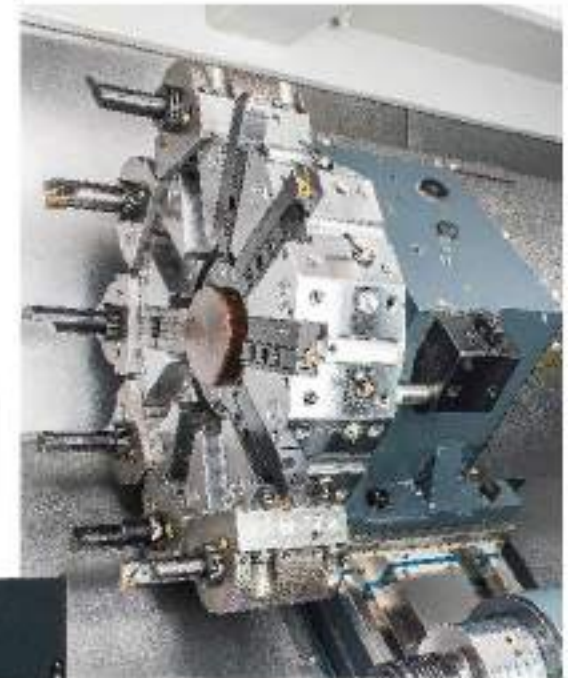
Alex-Tech self-made turret, Employ Japanese made curvic tooth clutch, hydraulic index- ing inrcinh motor.
